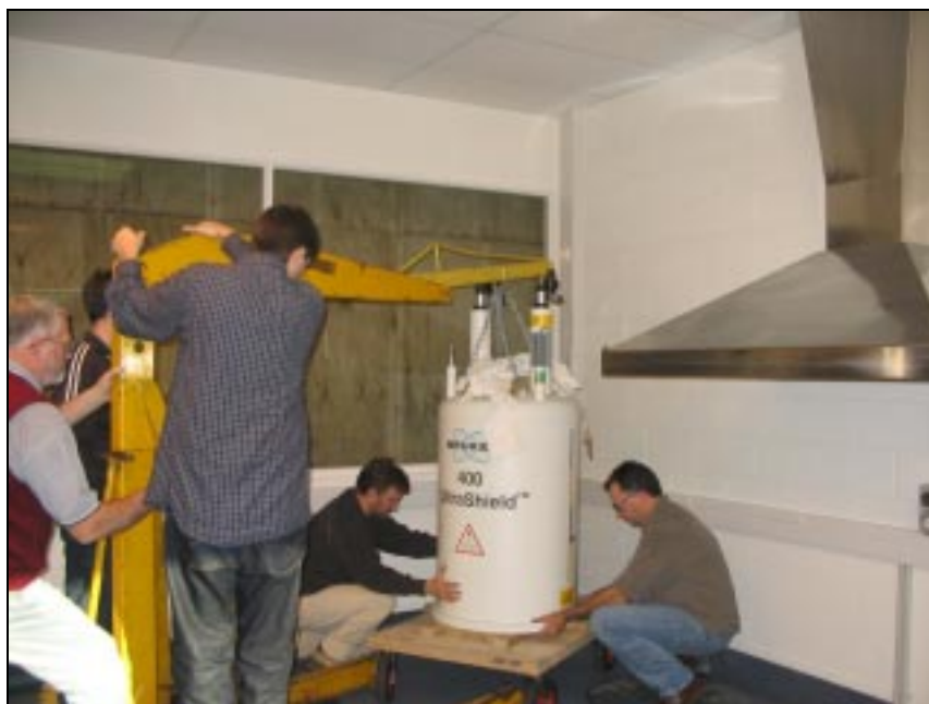
Take the weight, the 400 about to be lifted to mount the support legs
