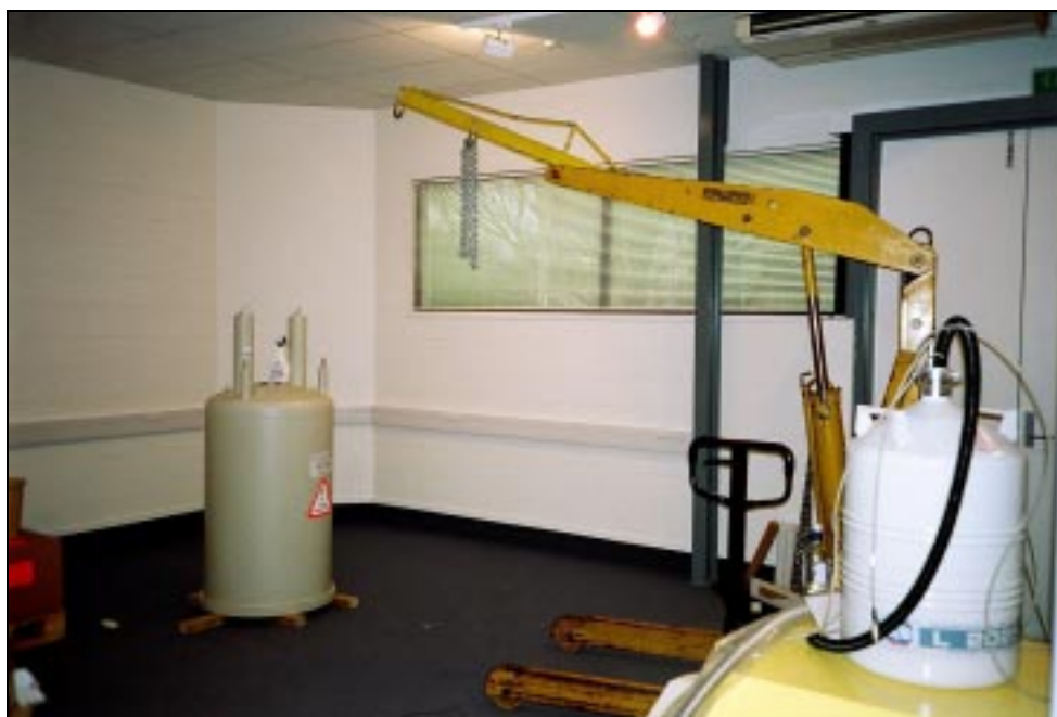
A legless 500 MHz magnet in the NMR Suite prior to being raised onto its support mounts
