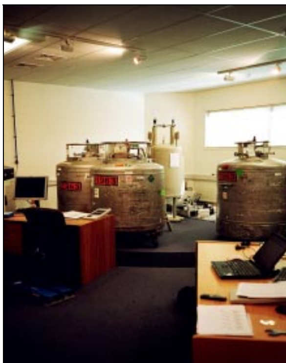
"Invasion of the Daleks" 500 magnet waiting its turn to be commissioned surrounded by liquid helium dewars
