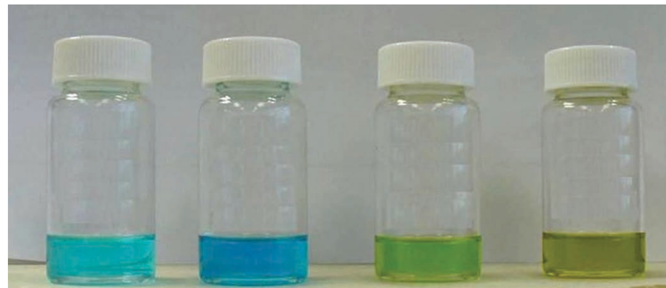
Polyphosphazenes in a variety of colours due to different metal-binding properties.
